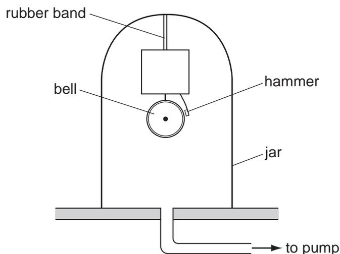
The pump is switched on and the air is removed from the jar. The hammer still hits the bell but the sound becomes quieter until it cannot be heard.
